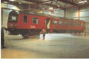
In this photo an expensive machine is being moved using an air bearing system. The yellow bearings underneath will support the weight of the load as they move across the facility floor.
