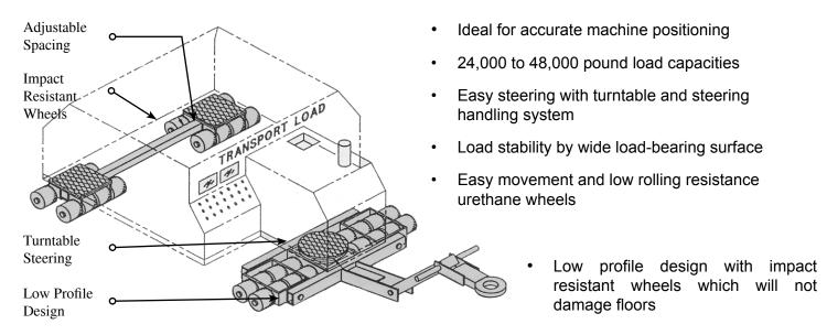
Typical drawings / diagrams showing turntable steering (SD) and rear adjustable (FX) dollies - sold as one of each in a set
