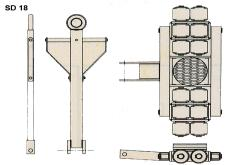
SD 18 - Steerable Dollies Maximum Load: 18,000 pounds Wheels: 12 each of 31/2" x 31/2" Non-skid turntable: 63/4" diameter Overall height: 41/4"
