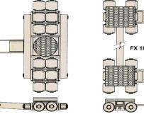
FX 18 - Rear Adjustable Dollies Maximum Load: 18,000 pounds Wheels: 12 each of 31/2" x 31/2" Non-skid load pad: 85%" x 51/4" Adjustable from: 20" to 63"
