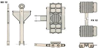
SD 12 - Steerable Dollies Maximum Load: 12,000 pounds Wheels: 8 each of 31/2" x 31/2" Non-skid turntable: 63/4" diameter Overall height: 41/4"
